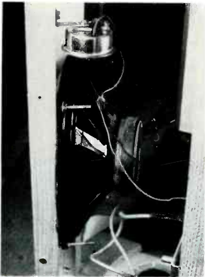
FIG. 36—SPEAKER AND HORN will later be covered by grille mounted over hole in skin.
