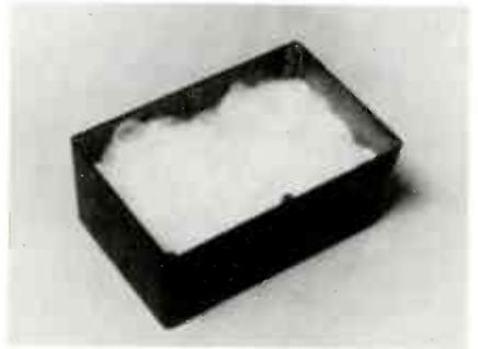
FIG. 7—POLYESTER PILLOW BATTING makes a good and inexpensive acoustic absorbent.
