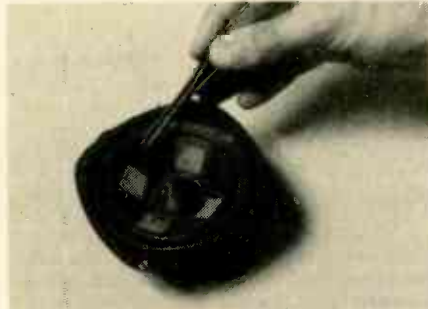
FIG. 8—FELT PADS cemented to bass/mid-range driver reduce "break-up."
