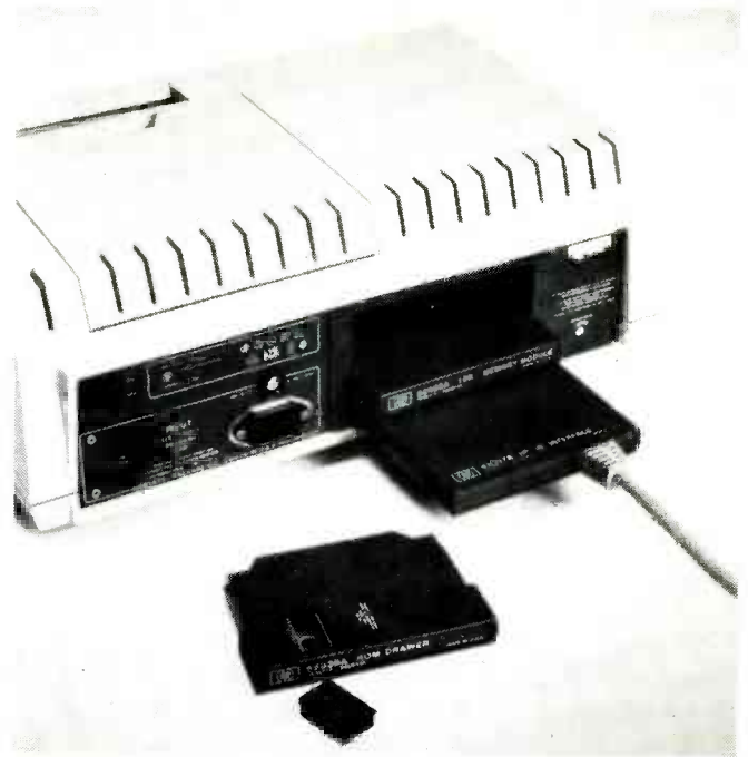
EXPANSION AND I/O modules plug into rear of HP-85.
