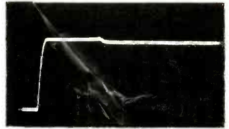
FIG. 10—SCOPE TRACE obtained in determining characteristic impedance of cable.
